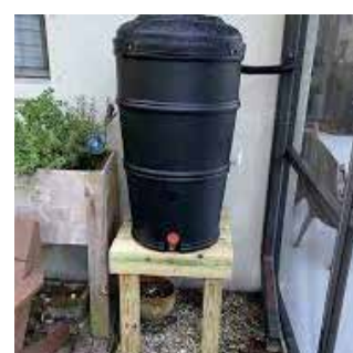
Rainwater tank. Image Source: NRCS
